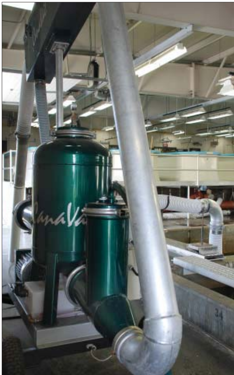
Left: This green machine sucks young chinook salmon from hatchery raceways and deposits them temporarily into stocking tanks.
