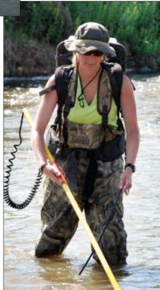
Below: Cari-Ann Hayer uses a backpack electroshocker to stun fish in the Wild Rice River.
