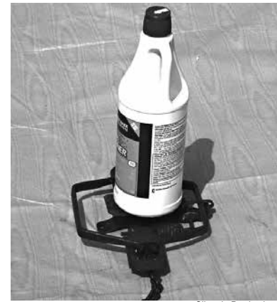
Plastic tube-like containers can be filled with sand or lead weights to create a certain known weight. Use this to test for the appropriate pan tension. Silvertip Productions
