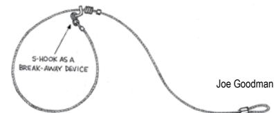
Joe Goodman Cable device with S-hook break-away device.
