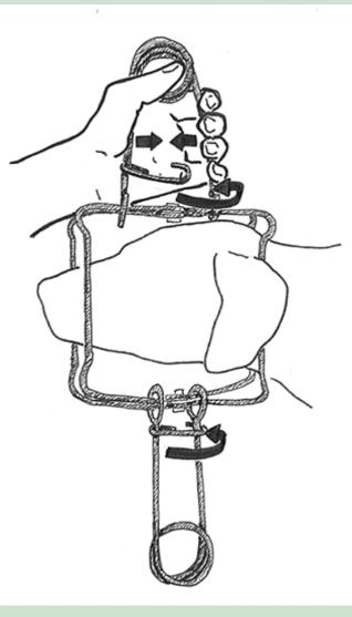
**Step 3:** Secure the safety lock, which keeps the spring compressed. Again, use both hands on each spring if necessary. This relieves the pressure from one side of the trap.
