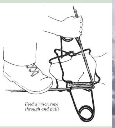
**Step 1:** Thread the rope through the large rings of one spring. The rings are located where the springs meet the rotating jaws.
