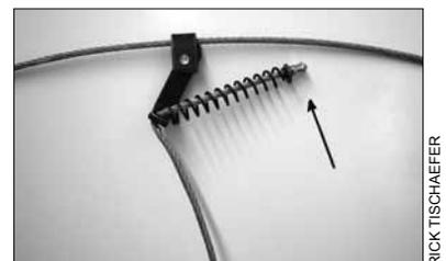
*An example of a release ferrule breakaway device.*
