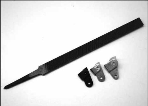
Cam locks can be purchased with and without teeth. A cam lock file is used to create or repair teeth on these locks.
