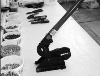
**A bench swagger is used to crimp aluminum ferrules. Use quality components and tools to make your cable devices.**
