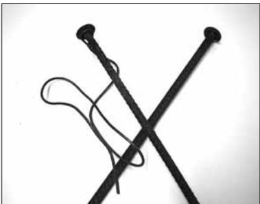
*Re-rod stakes used to cross stake for anchoring. Support wire is welded to one stake to provide a system to support the cable loop.*
